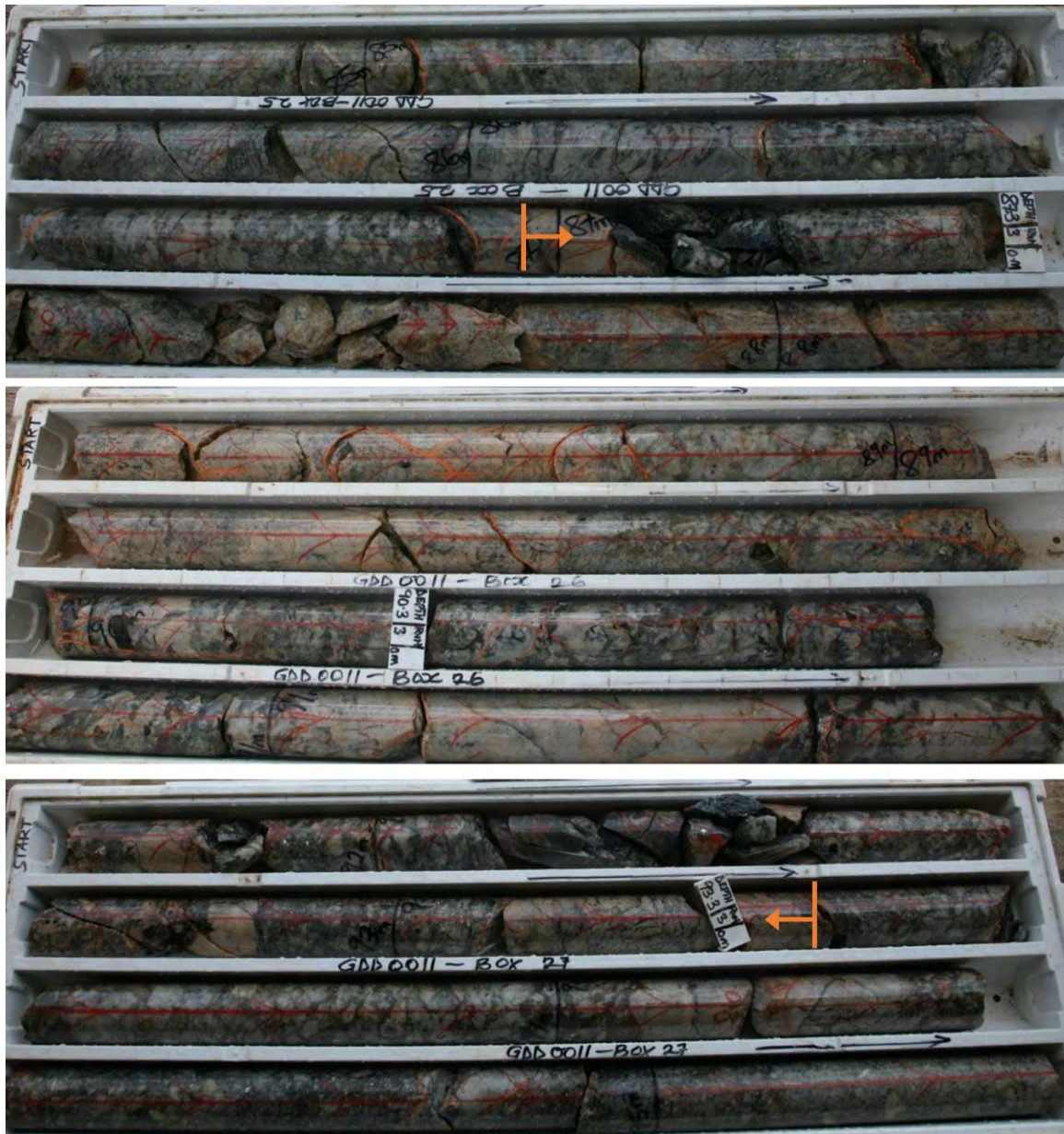
Figure 6-7: Chlorite-Muscovite-K Feldspar alteration zone in GDD0011 drill core between 86.90 m and 93.4 m
